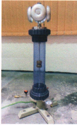
Figure 3. Set of test vessel for produce internal discharge.
