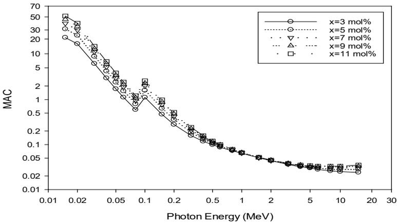
**Figure 1: Plot of mass attenuation coefficients (MAC) against photon energy of 20Li<sub>2</sub>O-xBi<sub>2</sub>O<sub>3</sub> (79-x)B<sub>2</sub>O<sub>3</sub>-1Ag glass system (x = 3,5,7,9 and 11 mol %)**
