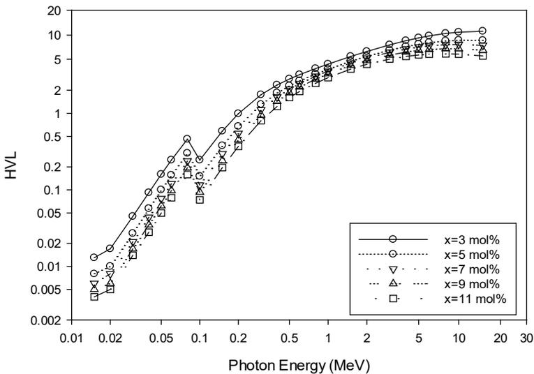
Figure 3: Plot of half value layer (HVL) against photon energy of  $20\text{Li}_2\text{O}-x\text{Bi}_2\text{O}_3-(79-x)\text{B}_2\text{O}_3-1\text{Ag}$  glass system ( $x = 3,5,7,9$  and  $11$  mol %)
