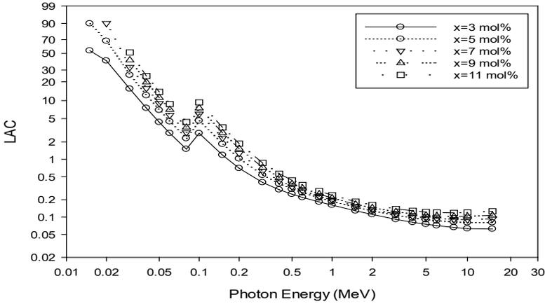
**Figure 2: Plot of linear attenuation coefficients (LAC) against photon energy of 20Li<sub>2</sub>O-xBi<sub>2</sub>O<sub>3</sub>-(79-x)B<sub>2</sub>O<sub>3</sub>-1Ag glass system (x = 3,5,7,9 and 11 mol %)**
