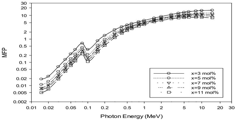
**Figure 4: Plot of mean free path (MFP) against photon energy of 20Li<sub>2</sub>O-xBi<sub>2</sub>O<sub>3</sub>-(79-x)B<sub>2</sub>O<sub>3</sub>-1Ag glass system (x = 3,5,7,9 and 11 mol %)**
