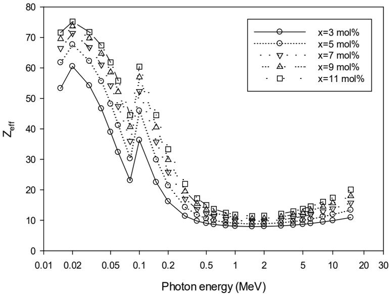
**Figure 5: Plot of effective atomic number ( $Z_{\text{eff}}$ ) against photon energy of  $20\text{Li}_2\text{O}-x\text{Bi}_2\text{O}_3-(79-x)\text{B}_2\text{O}_3-1\text{Ag}$  glass system ( $x = 3, 5, 7, 9$  and  $11$  mol %)**
