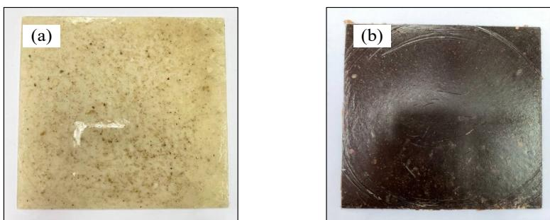
**Figure 1: Sample slabs of (a) PLA/PP polymer matrix and (b) DSF filled PLA/PP**
