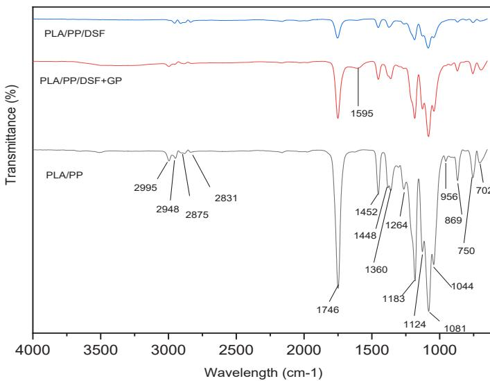
**Figure 2: Infrared Spectrum of PLA/PP, PLA/PP/DSF and PLA/PP/DSF+ GP composites**
