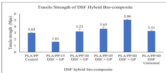
**Figure 3: Tensile strength of PLA/PP with different DSF loading treated and untreated with GP**
