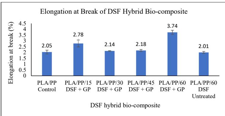
**Figure 5: Elongation at break of PLA/PP with different DSF loading treated and untreated with GP**
