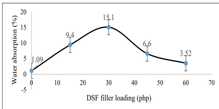
**Figure 6: The effect of filler loading on water absorption of PLA/PP/DSF bio-composites**
