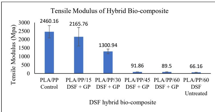
**Figure 4: Tensile modulus of PLA/PP with different DSF loading treated and untreated with GP**
