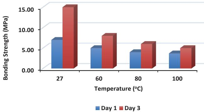
Figure 7: Bonding Strength Based on Different Curing Temperatures
