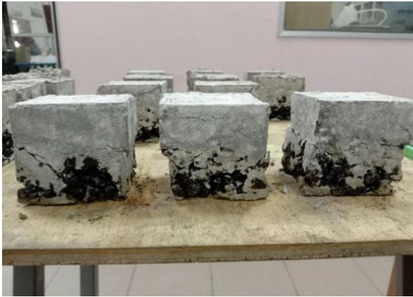
**Figure 5: Failure Mode C (Mix 3)**
