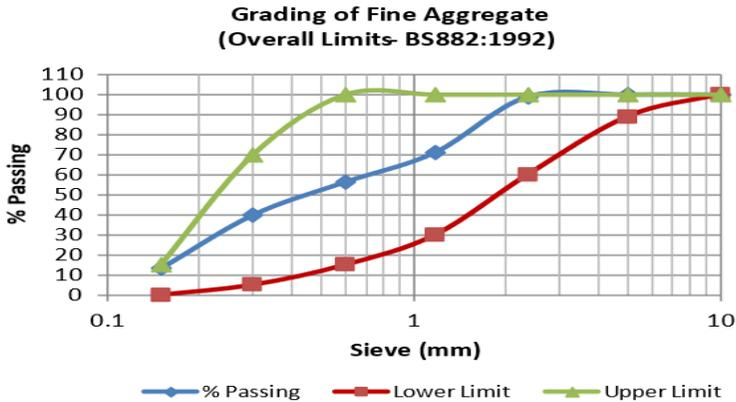
Figure 1: Particle Size Distribution of fine aggregates
