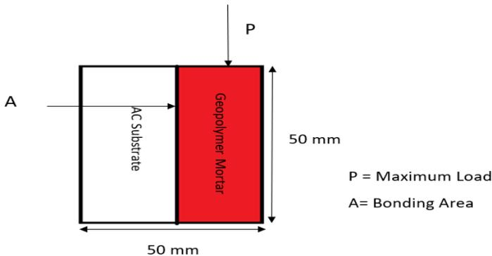
**Figure 2: Schematic Diagram of Testing**
