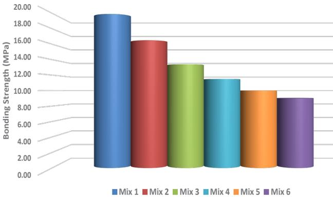
Figure 3: Bonding Strength based on different HCP content
