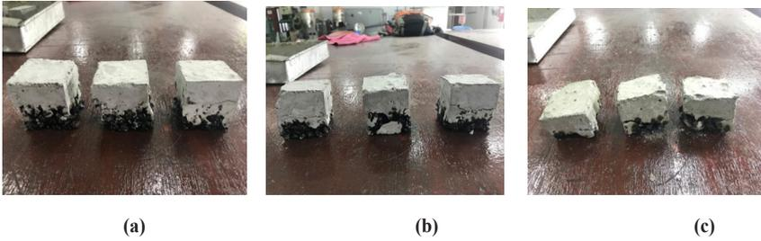
Figure 9: Curing at (a) 60 °C, (b) 80 °C and (c) 100 °C
