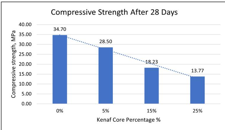
Figure 9: Compressive strength of kenaf core concrete after 28 days
