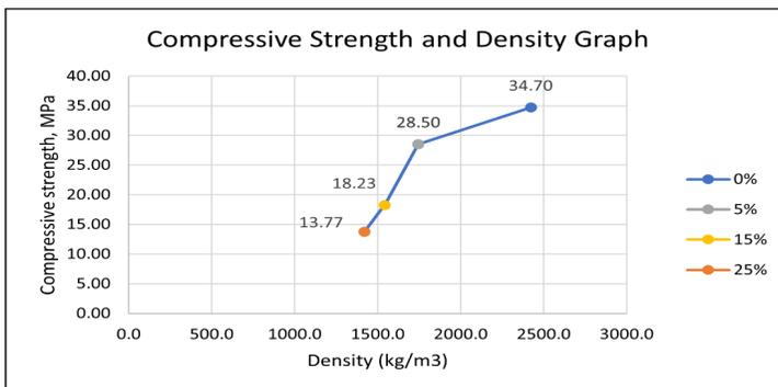
Figure 8: Compressive Strength versus Density graph
