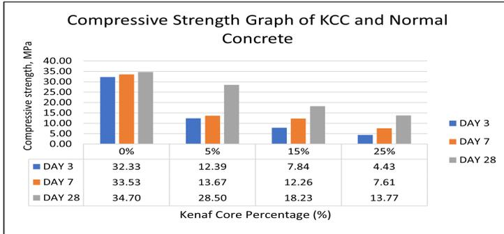
Figure 7: Compressive strength of kenaf core concrete and normal concrete
