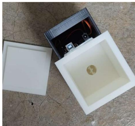
Figure 3. Top view of automatic fish feeder
