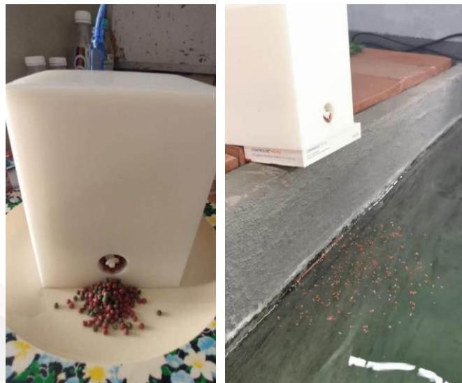
Figure 5. The amount of fish food dropped after the automatic fish feeder start functioning
