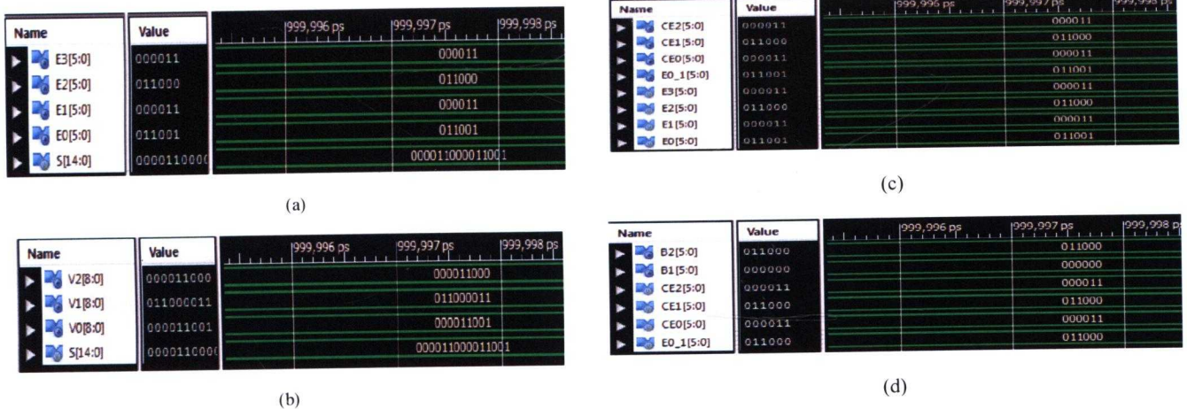
Figure 20: The Simulations Results Of The Modules Of The Checker And The Converters Of DNA Fragment Assembly With The Input Of 'ATATC': (a) The Result of the Edges Converter. (b) The Result of the Vertices Converter. (c) The Result of the Common Edges Checker. (d) The Result of the Branch Checker.
