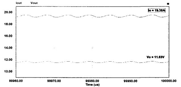
Fig. 15. Output voltage and output current at switching frequency of 90754.03507 Hz.
