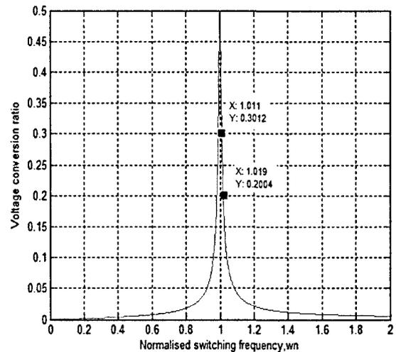
Fig. 7. Voltage conversion ratio curve at  $Q = 50$ .
