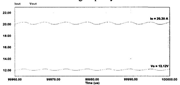
Fig. 19. Output voltage and output current at switching frequency of 91450 Hz.
