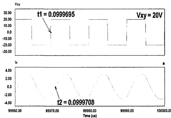
Fig. 11. Waveform of the voltage and current at the tank circuit element.
