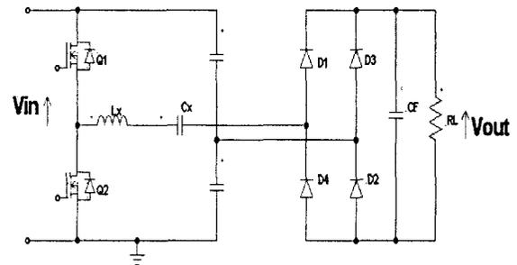
Fig 1. Half-bridge, series loaded resonant converter
