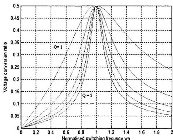
Fig. 4. Voltage conversion ratio for series-loaded resonant converter with  $Q = 1, 2, 3, 4, 5$ .
