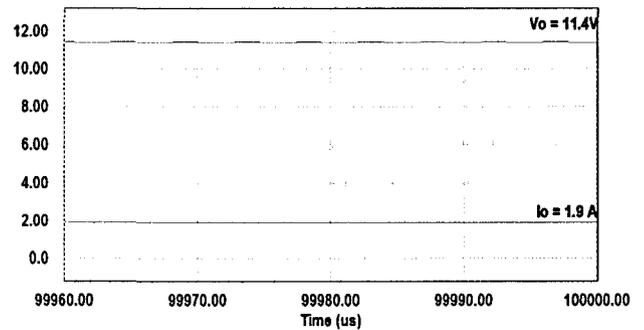
Fig. 12. Output voltage and output current at switching frequency of 107989 Hz.
