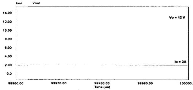
Fig. 13. Output voltage and output current at switching frequency of 106800 Hz.
