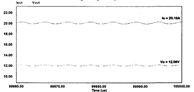
Fig. 16. Output voltage and output current at switching frequency of 90690 Hz.
