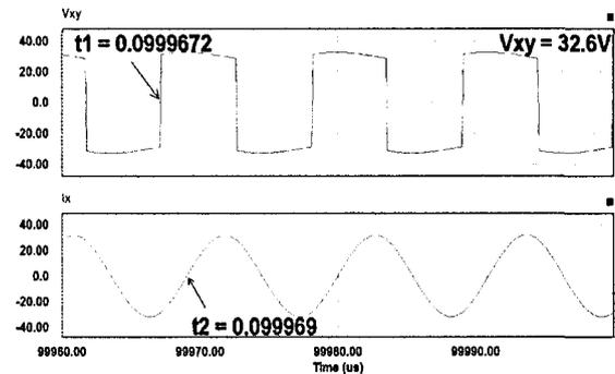
Fig. 20. Waveform of the voltage and current at the tank circuit element.
