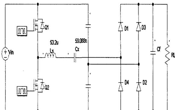
Fig. 5. Design circuit of SLR
