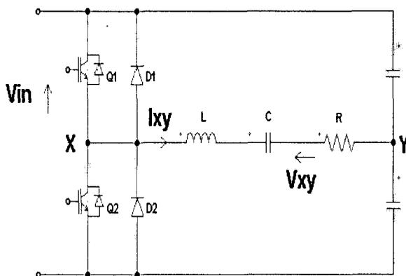
Fig. 3. Half-bridge and series L-C-R network.
