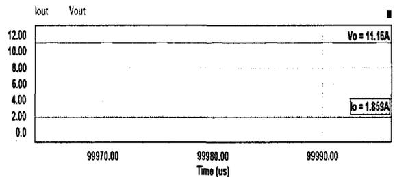
Fig. 9. Output voltage and output current at switching frequency of 100 kHz.
