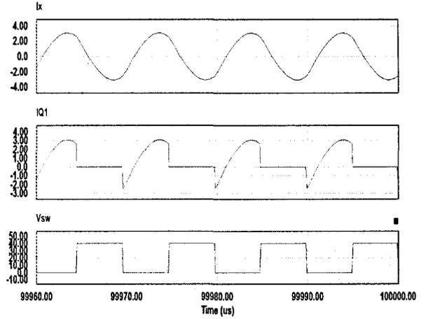
Fig. 8. Ideal resonant waveform of inductor current, drain current and switching voltage at frequency of 100 kHz from PSIM simulation.
