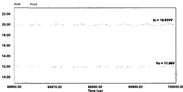
Fig. 18. Output voltage and output current at switching frequency of 91472.1688 Hz.
