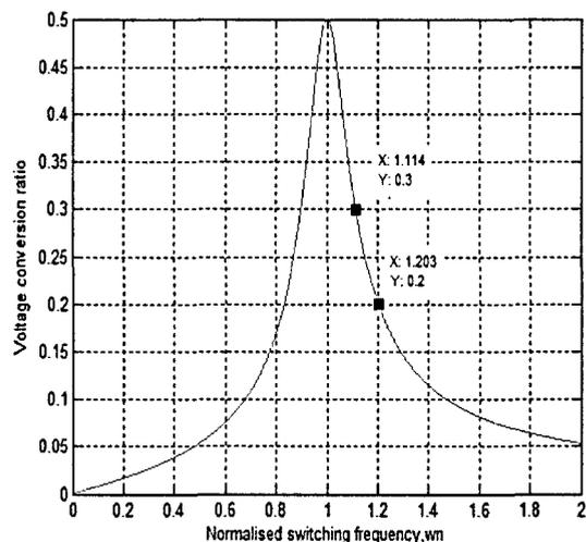
Fig. 6. Voltage conversion ratio curve at  $Q = 5$ .
