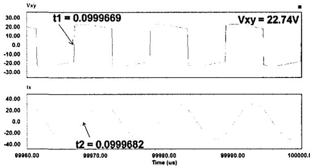
Fig. 17. Waveform of the voltage and current at the tank circuit element.
