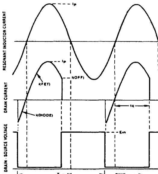
Fig 2. Ideal resonant converter waveforms.
