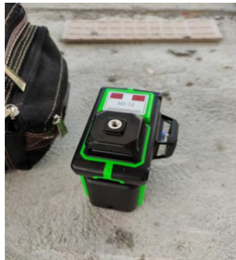
Figure 3.3.3(1) The laser worker used to help marking height for installation of the ceiling
