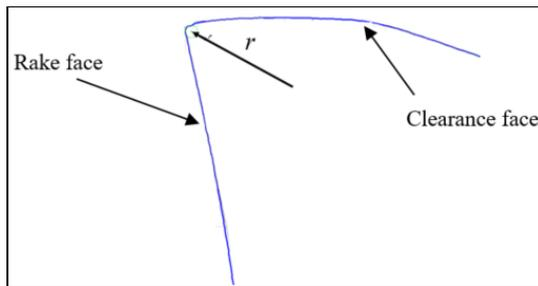
Figure 9: Profile of cutting edge radius measured from the software available in Keyence VHX-6000 digital microscope
