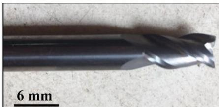
Figure 1: Carbide milling cutter with three-helix cutting edges
