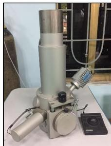
Figure 3: SEM machine referenced under JEOL-JSM 5410 LV
