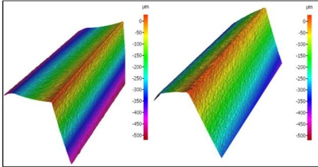
Figure 10: Cutting edge form after machining at the length of; (a) 15 cm, and (b) 300 cm with feed speed of 500 mm/min and spindle speed of 8000 rpm
