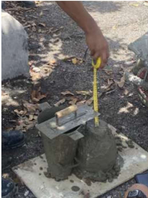
Figure 3.19: The Assistant Engineer measured the slump test
