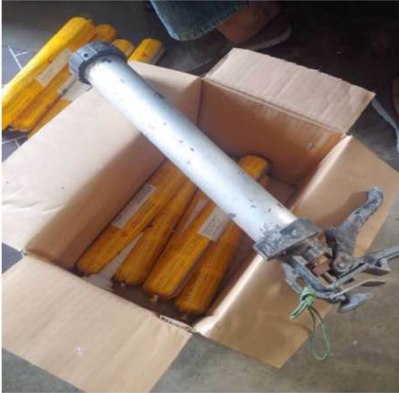
Photo 3.35 Pointing Mortar Gun Tile Grout that fill in with SikaBond
