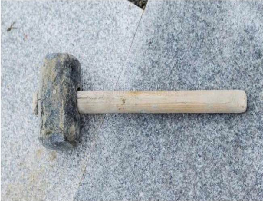
Photo 3.27 Rubber Hammers to make sure the Surface Tiles Level
