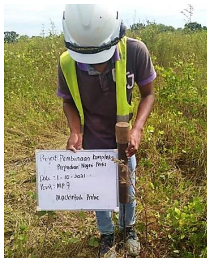
Figure 3.16 conducted Mackintosh Probe Test
