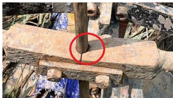
Figure 3.21 gap in lifting handle
