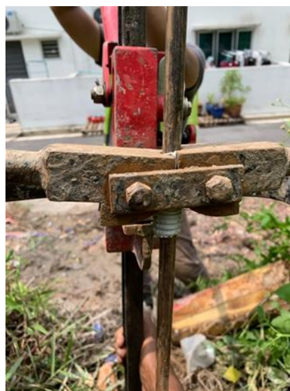
Figure 3.23 wrapping penetration rod with water host
