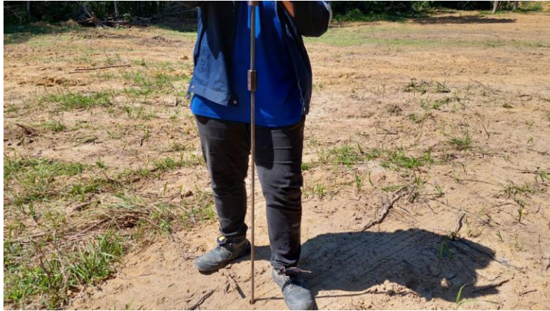
Figure 3.14 raising mackintosh probe hammer
