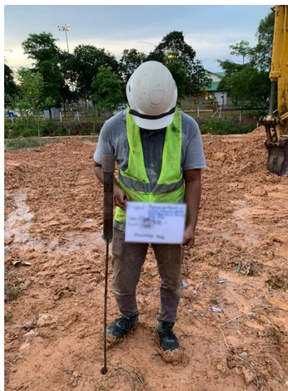
Figure 3.15 conducted Mackintosh Probe Test
