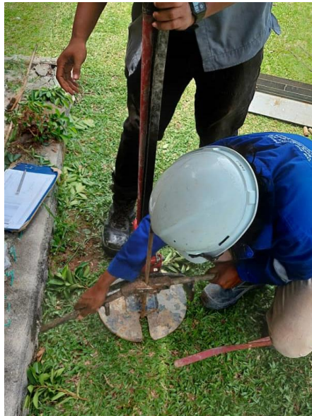
Figure 3.22 pulling out penetration rod using modified jet
