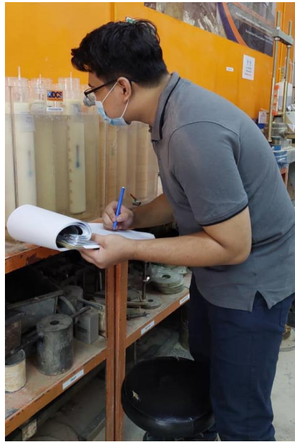
Figure 3.6 taking hydrometer reading
