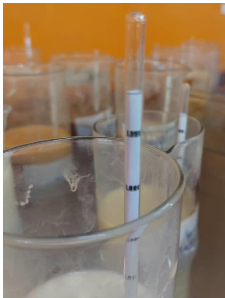
Figure 3.7 Hydrometer test reading
