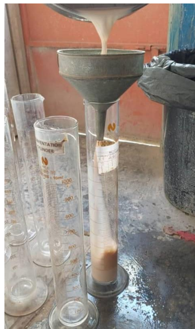
Figure 3.5 pouring dissolve silt and clay into measuring cylinder
