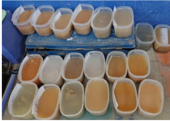
Figure 3.4 soaking sample with Sodium Hexametaphosphate
