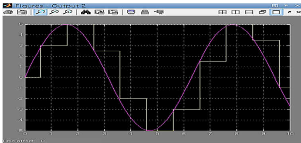
Figure 4.2 Combination of sine wave and PAM signal display in output 2 scope.
