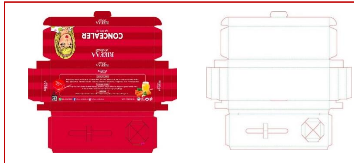
Figure 1. Innovation Cosmetic Packaging Technical Drawing
