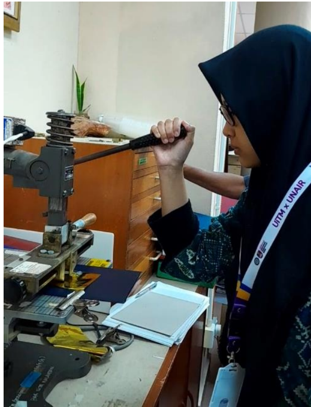
Figure 3.66 Printing the name on the hard cover
