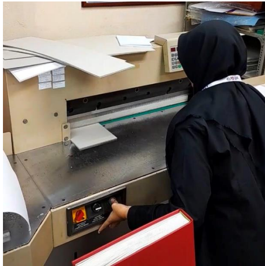
Figure 3.63 Cutting the hard cover
