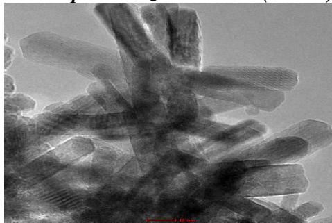
Pd doped SnO 2 - HRTEM (10 nm)
