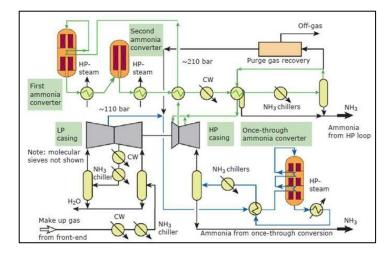
The PFD of the three-bed ammonia reactor from the Uhde process dual-pressure ammonia synthesis based on SAFCO IV ammonia plant in Al-Jubail, Saudi Arabia
