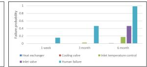
Failure probability graph of the safety barriers for three time-slices
