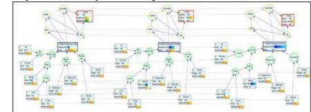
Reactor overpressure of ammonia reactor for three time-slices
