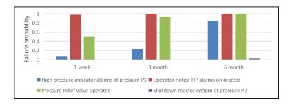
Conventional risk analysis of reactor overpressure of the ammonia reactor for comparison study
