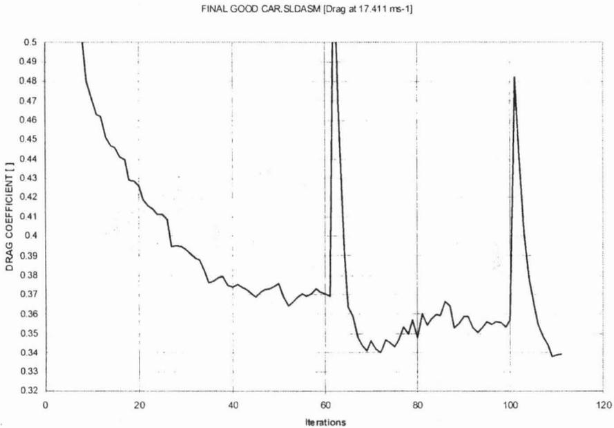
Fig. 5: The Drag Coefficient value Calculated via COSMOS-FLOWWORKS.
