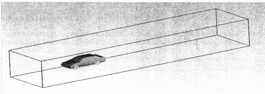
Fig. 2: The Computational Domain and the CAD Model Testing in COSMOS-FLOWWORKS
