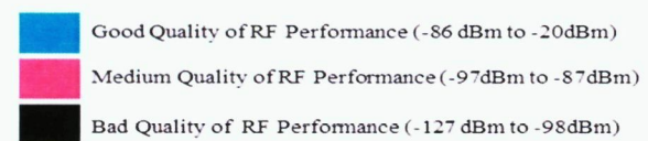
Figure 8 : RF Measurement Indicator
