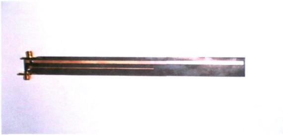
Figure 14: Microstrip of Reflectometer
