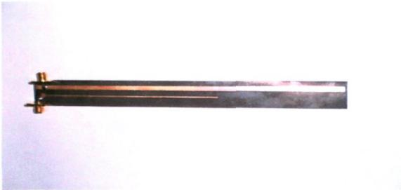
Figure 14: Microstrip of Reflectometer
