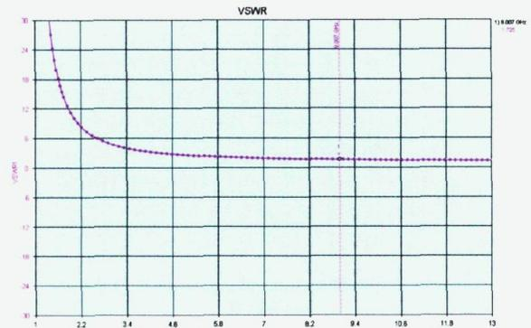
**Figure 6: Graph of voltage standing wave ratio (VSWR)**
