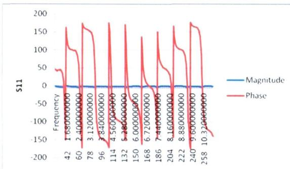
Figure 15: Graph of reflection coefficient versus frequency for short circuit
