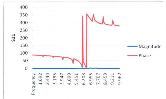
Figure 16: Graph of reflection coefficient versus frequency for open circuit
