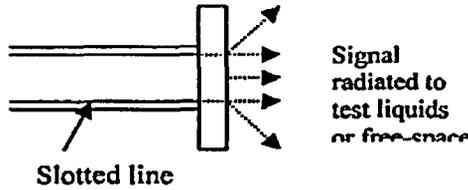
Figure 1: Arrangement for radiating liquid [1]
