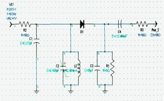
**Figure 4: An open circuit of slotted line operates at 9 GHz**
