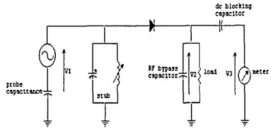
Figure 3: A slotted line detector equivalent diagrams [5]
