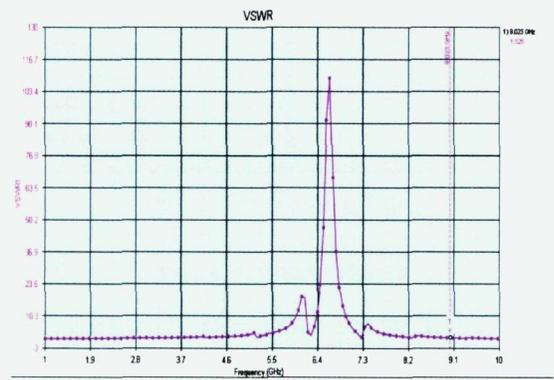
Figure 12: Input VSWR versus frequency response of distributed element after optimization
