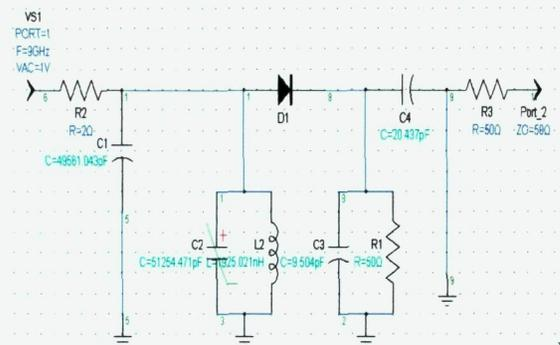
**Figure 7: A short circuit of slotted line operates at 9GHz**
