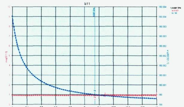
**Figure 8: Graph of reflection coefficient ( $S_{11}$ ) versus frequency**
