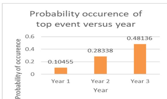
Figure 2: Probability occurrence of top event (Chlorine gas release from drum) versus year
