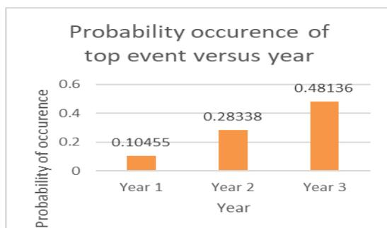
Figure 2: Probability occurrence of top event (Chlorine gas release from drum) versus year
