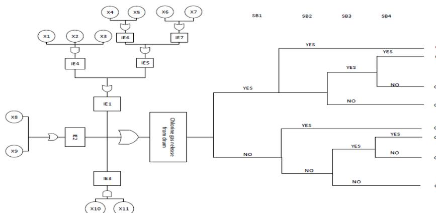
Figure 1: Accident scenario modelling of chlorine gas leakage from drum using Bow-tie approach
