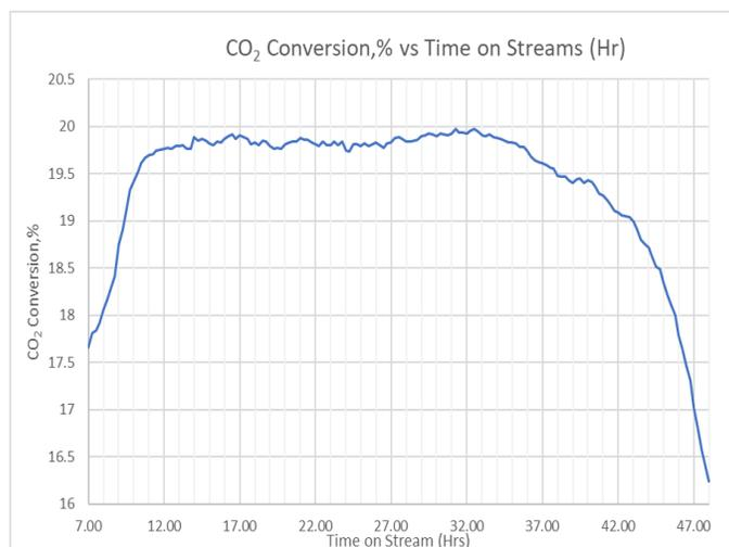
Figure 3 The Deactivation Trend on 47h of Reaction
