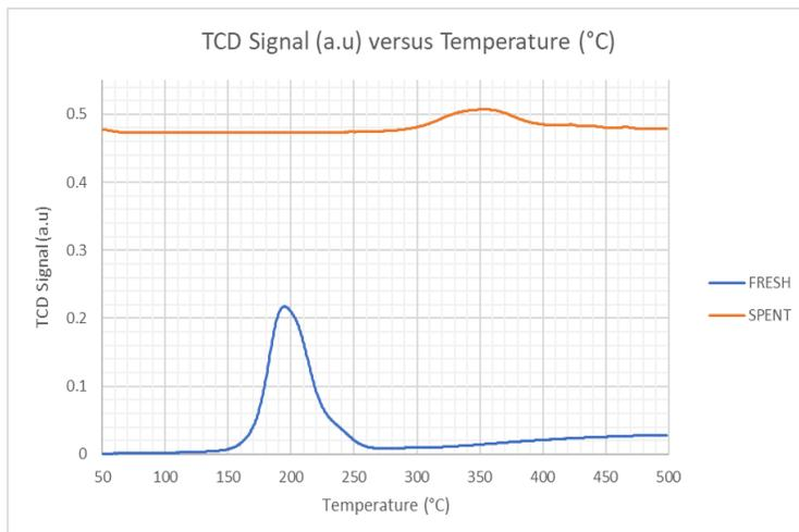
Figure 2 TPR Profile for fresh and spent Cu/Zn/Al/Zr catalyst sample
