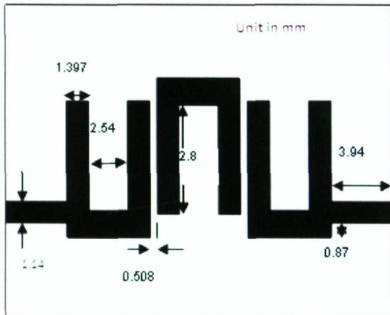
Fig.2: The dimension after last optimizing
