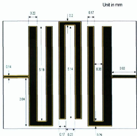
Fig.4: The dimension hairpin on metamaterial substrate
