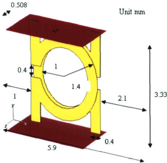
Fig 1: A unit cell of omega structure
