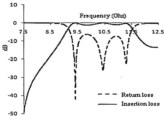
Fig.8: The graph of S11 and S21 for conventional
