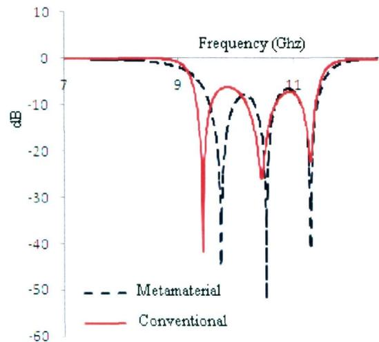
Fig.7: The graph of S11 for conventional and metamaterial filter
