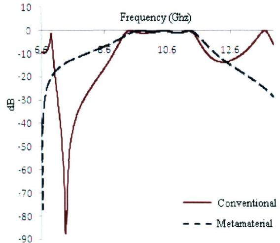
Fig.6: The graph of S21 for conventional and metamaterial filter
