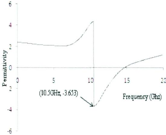
Fig.5: A Graph permittivity versus frequency
