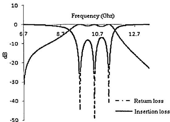
Fig.9: The graph of S11 and S21 for metamaterial July 200
