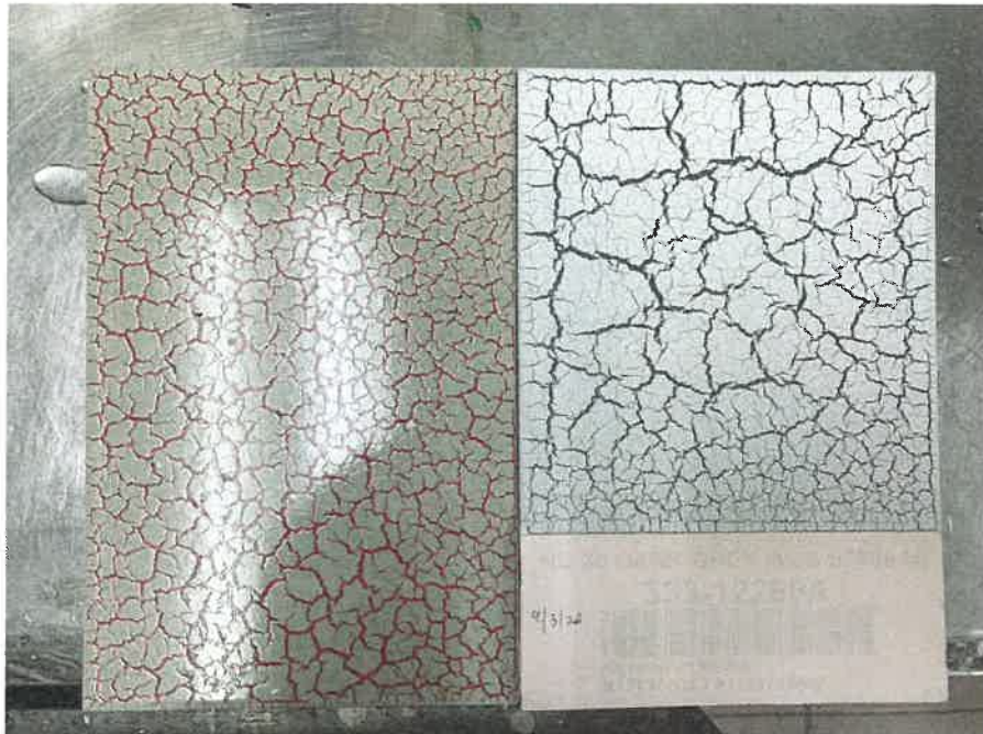
Figure 4.2.7 Result of Cracking Top Coat Panel
