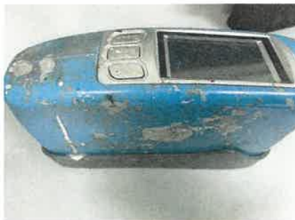
Figure 4.2.6 Gloss Meter to Measure Gloss
