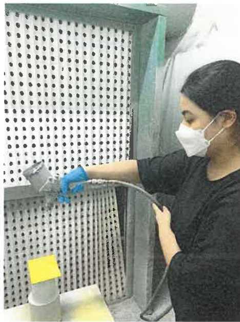
Figure 4.2.5 Spray Panel Using Spray Gun
