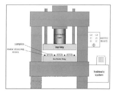
Figure 4.9 Working Princple of Hot-press
