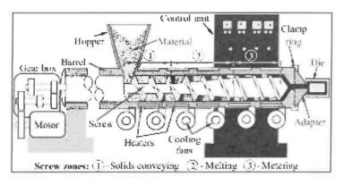
Figure 4.7 Single Screw Extruder Diagram Working Principle
