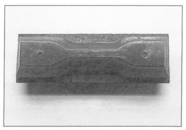
Figure 4.14 Dumbbell shape ASTM D638 Type IV
