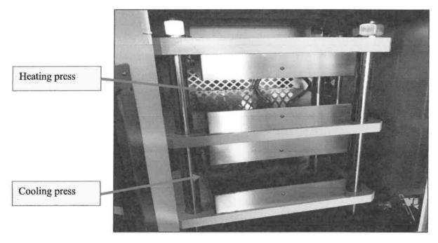
Figure 4.11 Hot compression moulding machine with heating press system
