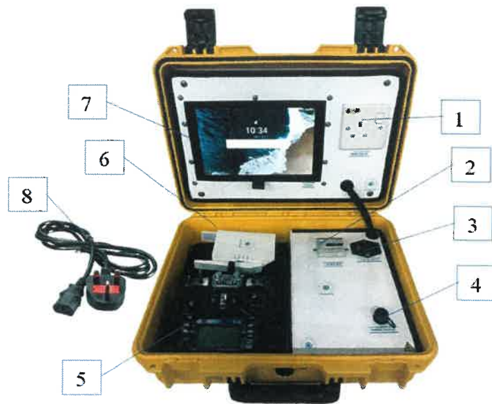
Operation Control Unit (OCU) interior consisting a power supply, remote control, wireless adapter and an Android Tablet
