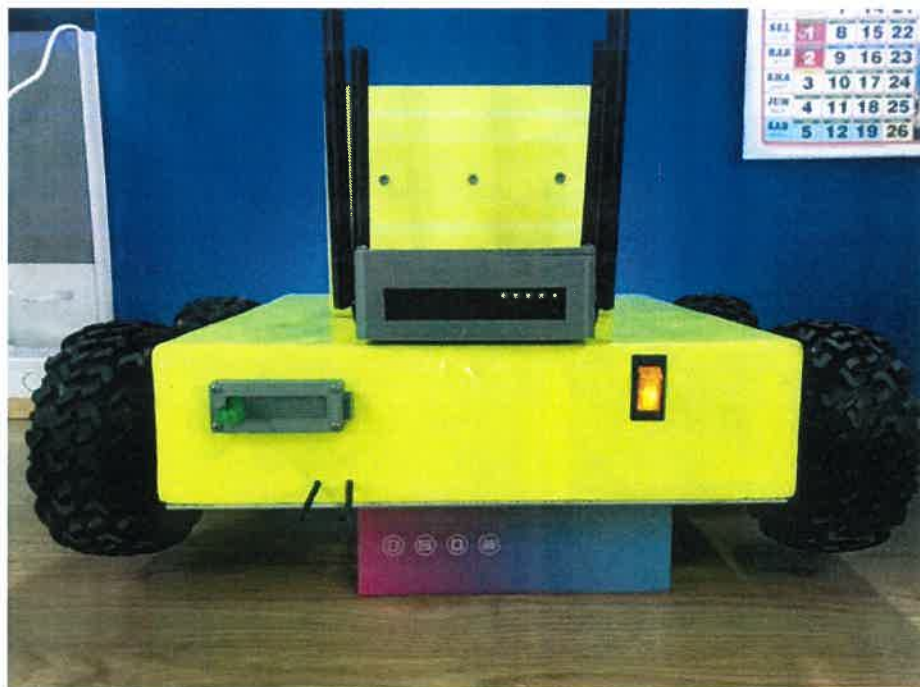
This figure above is called Roam where it is used inside a storage tank or a reactor. As shown above, it contains a battery that can lasts 4 hours, waterproof-sealed charger, power button, 360 camera and it moves with four wheels. These four wheels are made with strong rubber with grip patterns to ensure the utmost grip at harsh conditions especially when there is residue present at the particular equipment. It is controlled using a remote control shown. Findings were captured using the 360 camera and livefeed is uploaded using an Internet connection.
