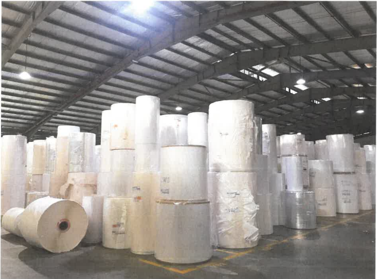
Figure 2.7: Jumbo (Label stock) at warehouse
