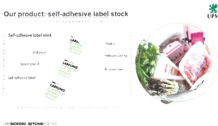
Figure 2.5: Structure of Label stock
