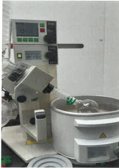
Figure 2: the water vapor to extract the standards solutions from 80 ml to 5 ml concentrated
