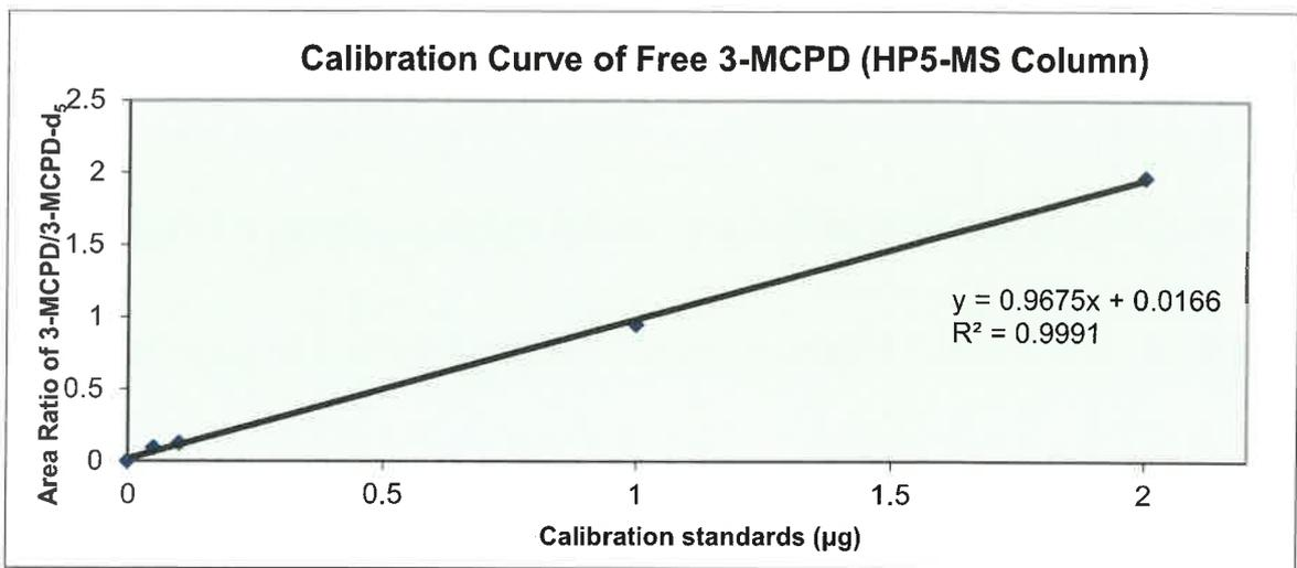
Figure 4.3.2: Calibration curve of free 3-MCPD
