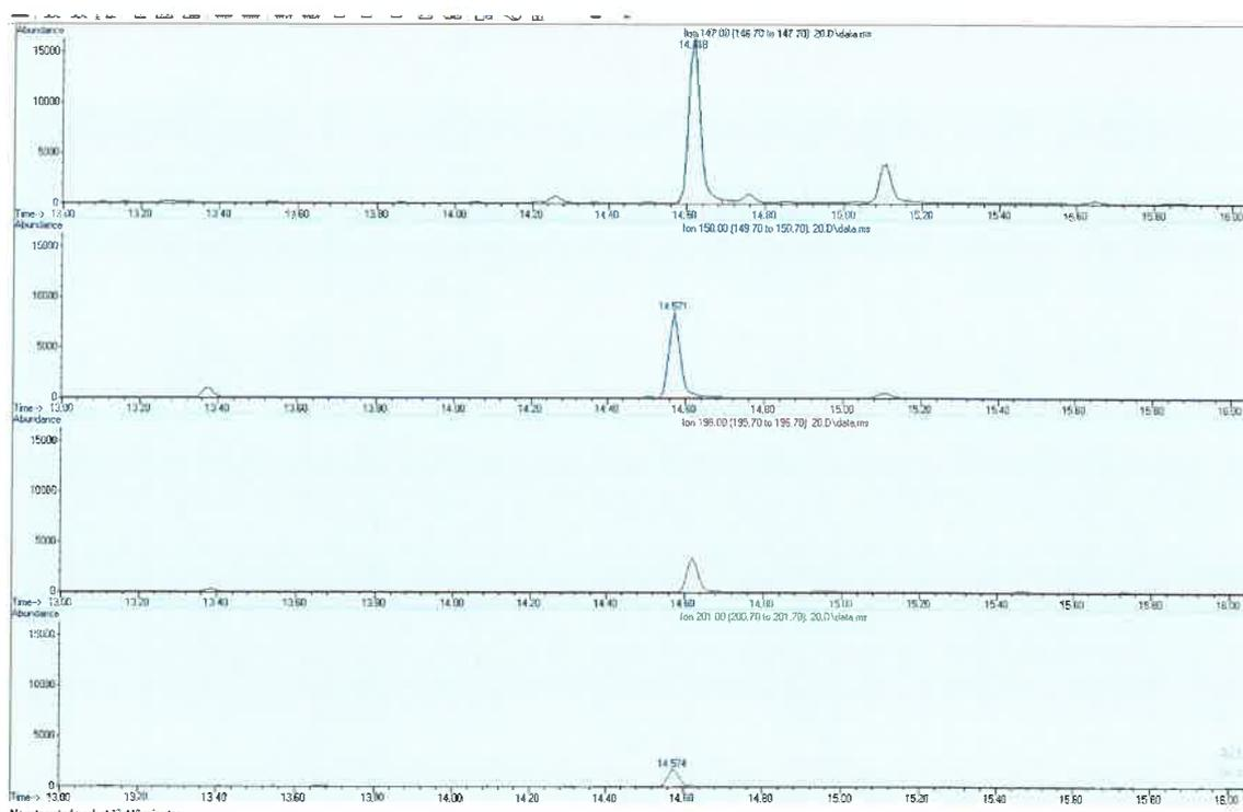
Figure 4.3.1: the peak of 3-MCPD and 3-MCPD-d5 for calibration standard of 2.00 µg/ml.
