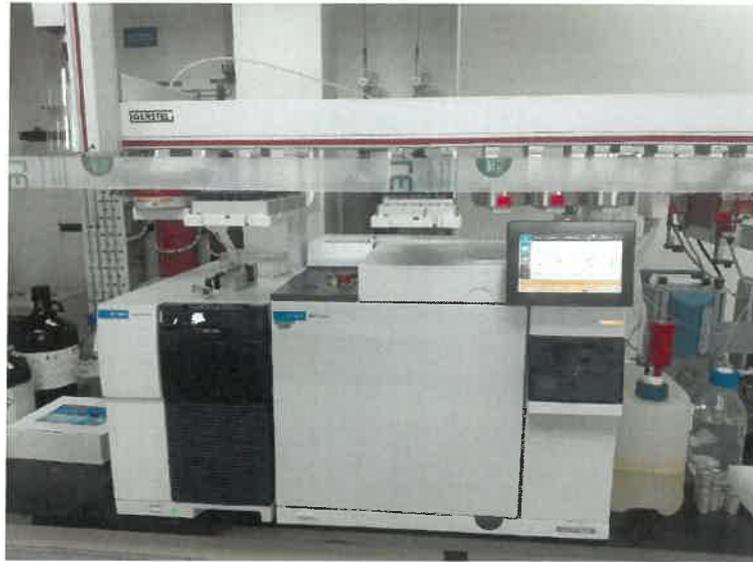
Figure 4.2.4: the GC-MS instrument
