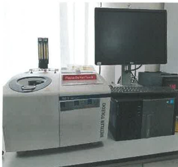
Figure 7 Differential Scanning Calorimeter (DSC3)
