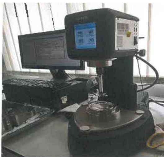
Figure 2 HAAKE Viscometer IQ - Rheometer
