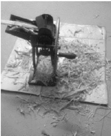
**Figure 1:** Bagasse From Dry Sugarcane was Minced into Small Pieces
