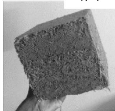
**Figure 5:** The Bio-Brick Was Given a Month to Dry in The Air
