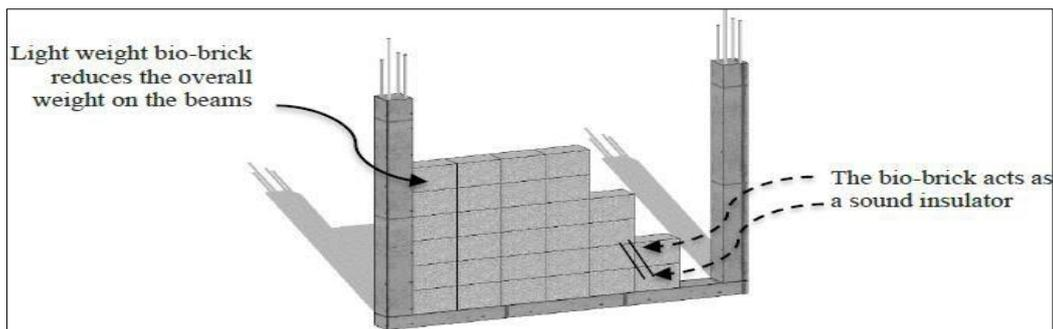
**Figure 7:** Material for column-and-beam structures' filler walls
