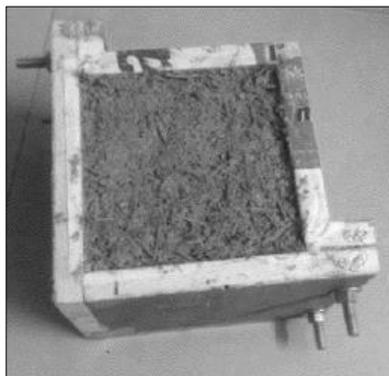
**Figure 4:** In the mould, the mixture is appropriately pressed down.
