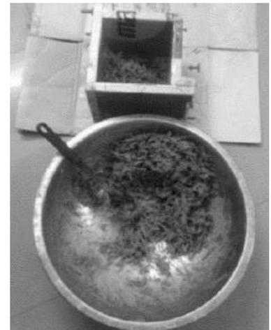
**Figure 3:** Stone dust, Lime, Water, and Chopped Bagasse Were Appropriately Combined
