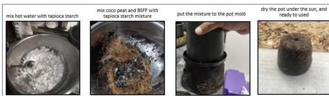
Figure 2: Process Making the Pot
