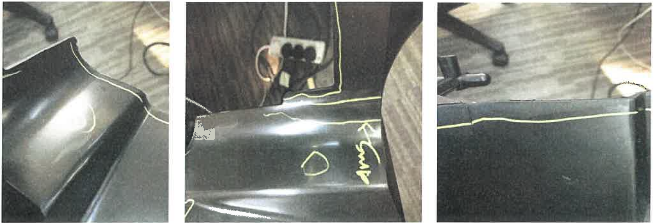
FIGURE 13: Defects (left to right) sinkhole, scratches, runner-up
