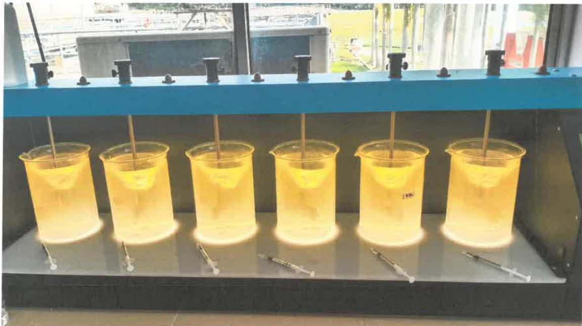
Figure 4.2.1 Jar Test at Sungai Linggi Water Treatment Plant
