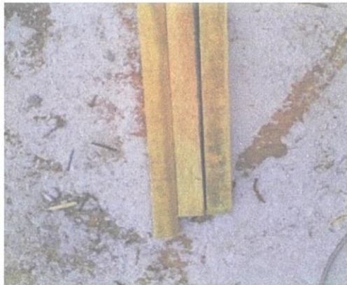
Photo3.19 Not accurate when cutting material.
