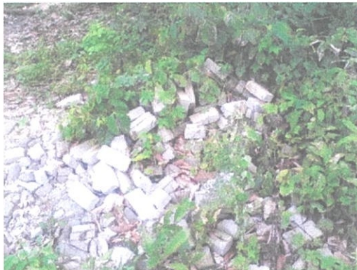
Photo 3.7 Brick left too long.
