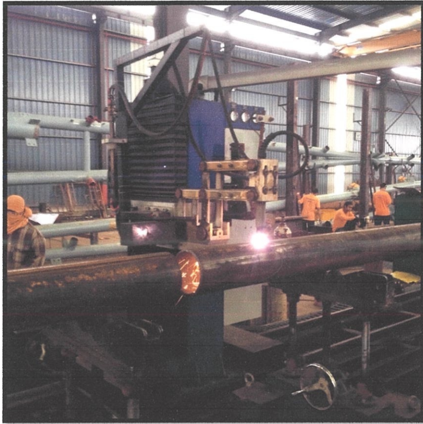
Photo 3.5 Cutting by Computer Numerical Control Profile Cutting (CNC) Machine.
