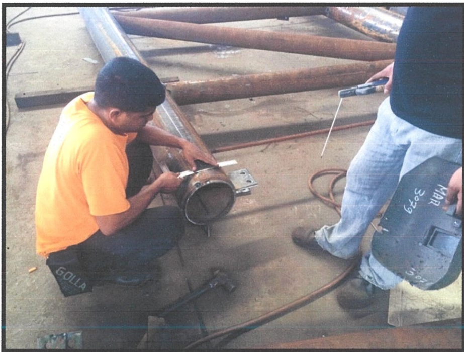
Photo 3.4 Marking process must be done to prevent from wrong cutting of the raw material.
