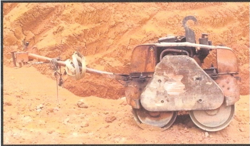
Photo 3.4 Roller Compactor 2 ton
