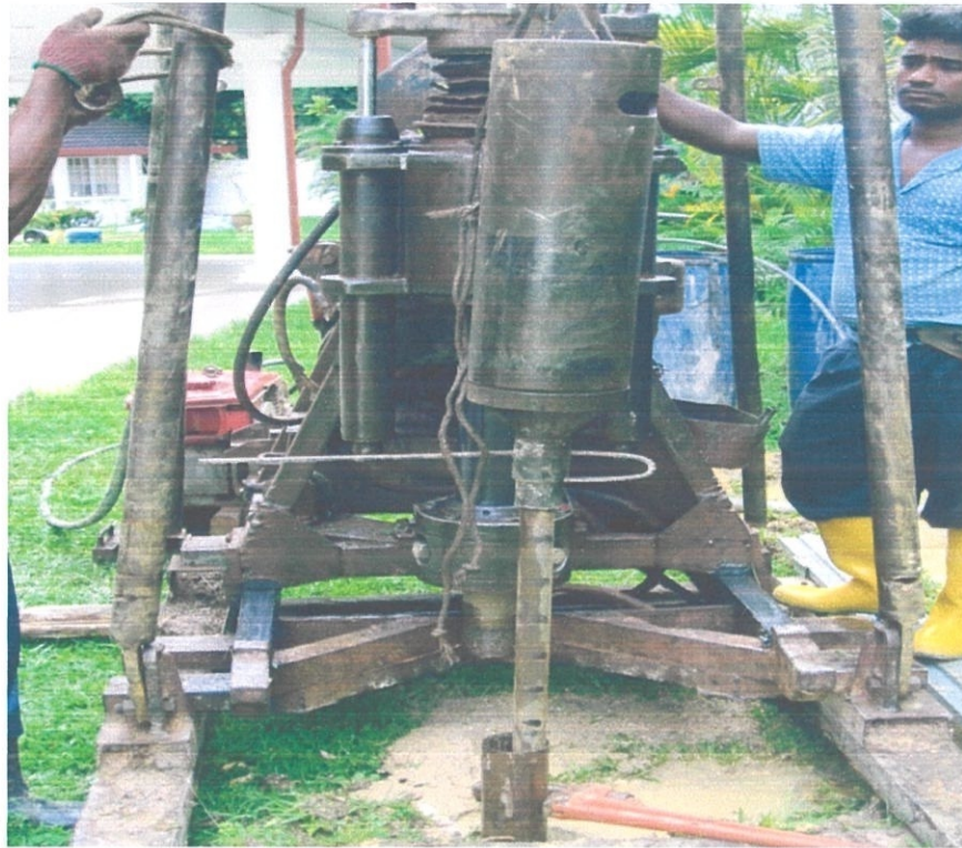
Figure 4.9: 65kg automatic trip hammer free-falling through a height of 760mm.
