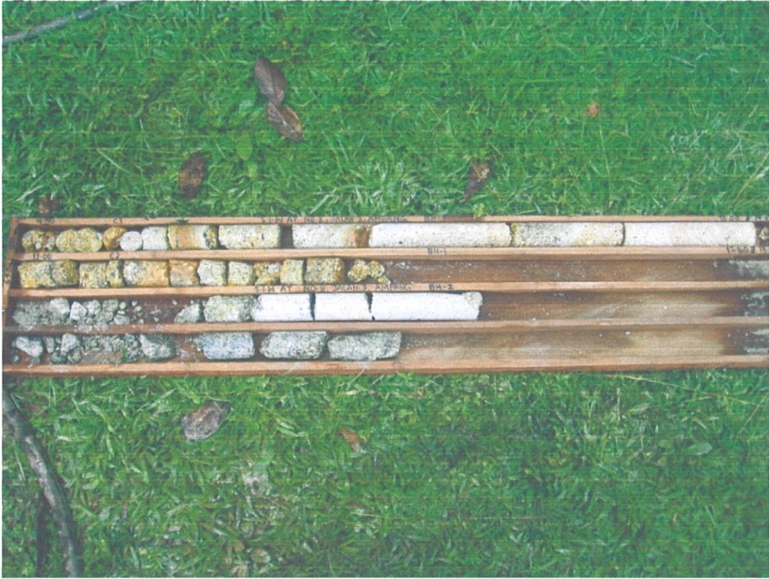
Figure 4.9.5: Result/Sample that are taken by using Core Barrel
