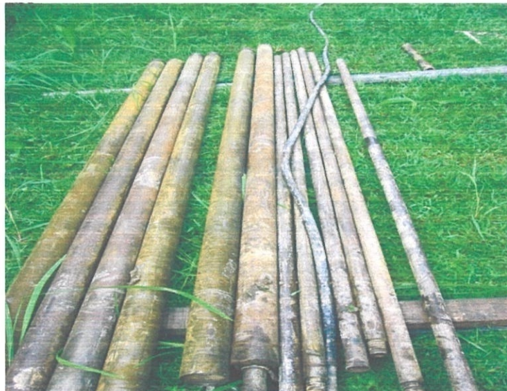
Figure 4.2: HW casing (101mm I.D) and NW casing (76mm I.D)
