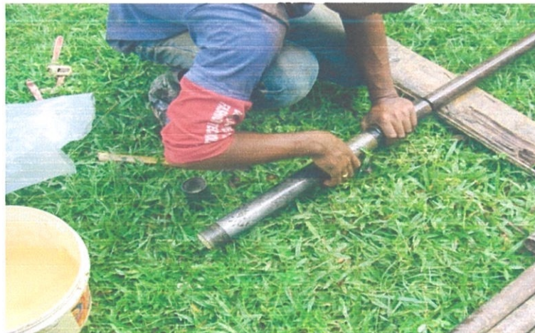
Figure 4.9.2: SPT that are just taken out from the hole
