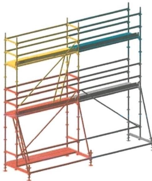
Figure 10 : Prefabricated Scaffolding System
