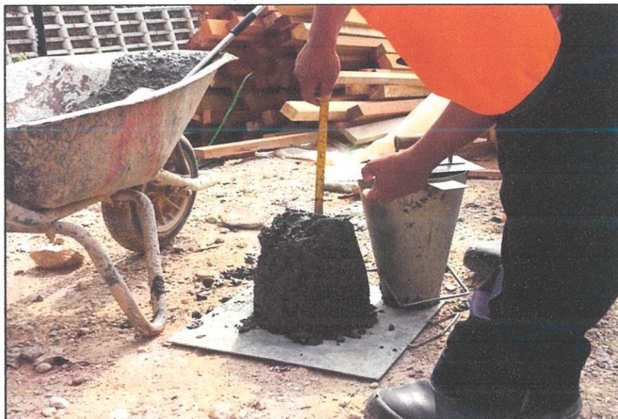
Photo 3.9: The slump of concretes is measured.
