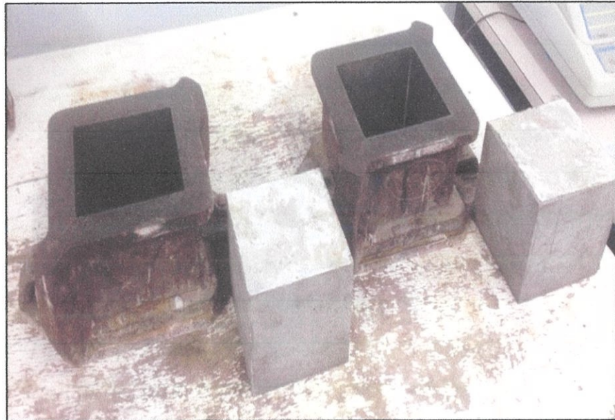
Photo 3.15: The cube is dismantled from mould.
