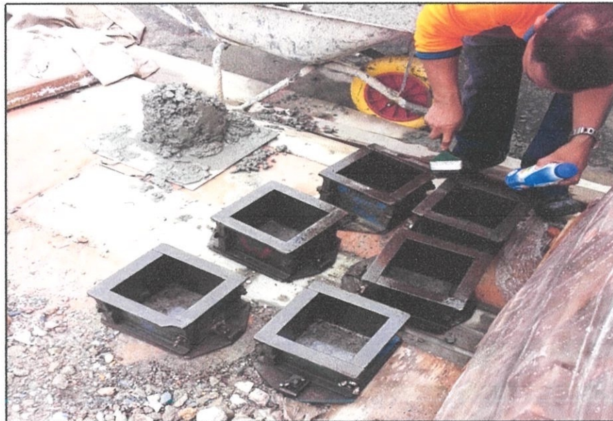
Photo 3.10: The oil is put on the mould and base plate.
