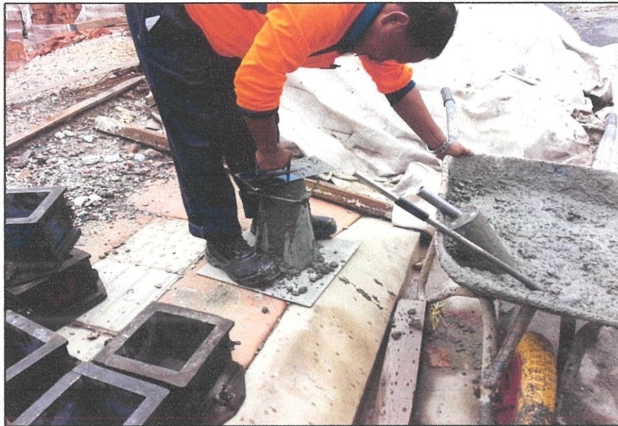
Photo 3.6: The top surface of frustum is struck off with the scrapper.
