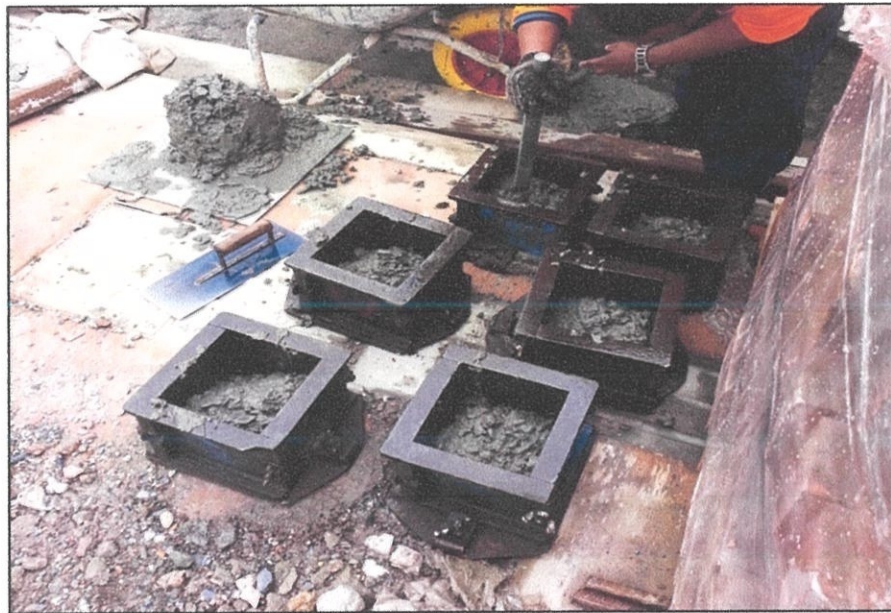
Photo 3.12: The concrete is compact for 25 times.
