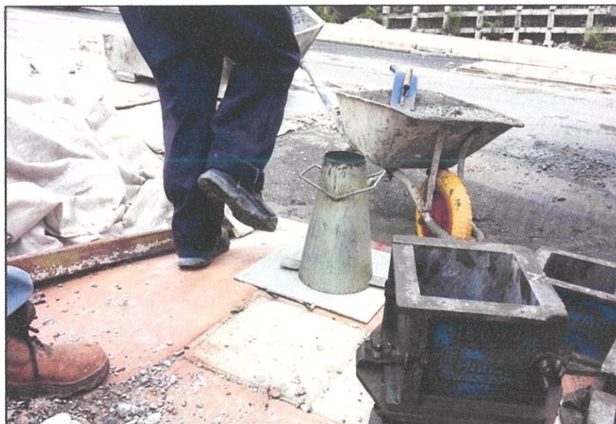
Photo 3.3: Frustum is place on the base plate.
