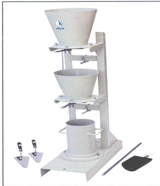
Figure 3.2: Compact factor apparatus.
