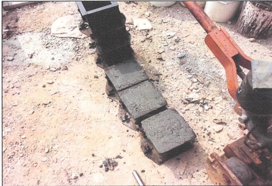
Photo 3.13: Struck off and smoothen the upper surface of mould.
