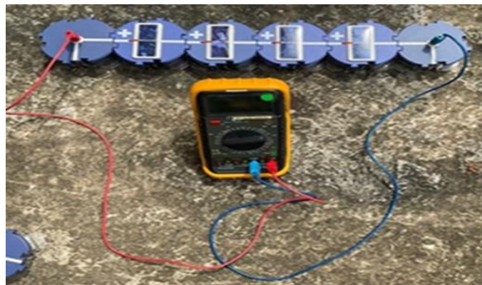
Figure 2: Solar panel cells arranged in a series circuit
