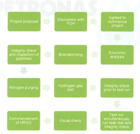
Figure 37 Flow chart for Reinstating H2RG system supply from PDH project
