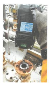
Figure 38 Gas testing indicates zero H2 during both nitrogen purging and leak test.
