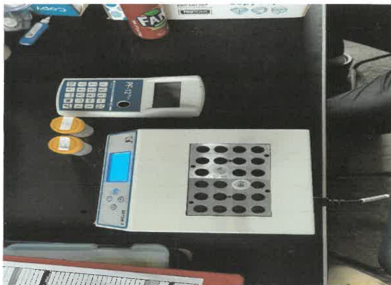
Figure 17 COD test equipment
