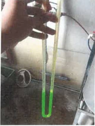
Figure 13: Changing the manometer liquid.
