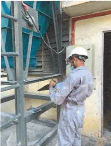
Figure 5: I record the reading. Figure 6: The pressure drop reading and compressed air pressure reading.
