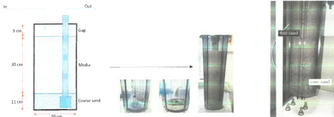
Figure 15. System Setup of Sand Filtration
