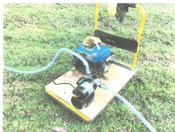
Figure 11. Generator and water pump used for fill up floating wetland holding tank
