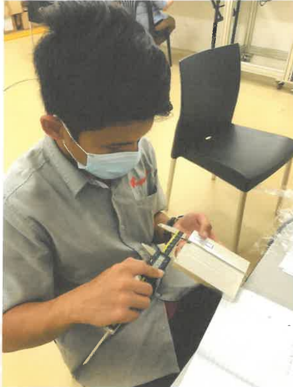
Figure 32: A picture of an Intern Measuring the Jig that just Arrived for the use of Felt Measurement
