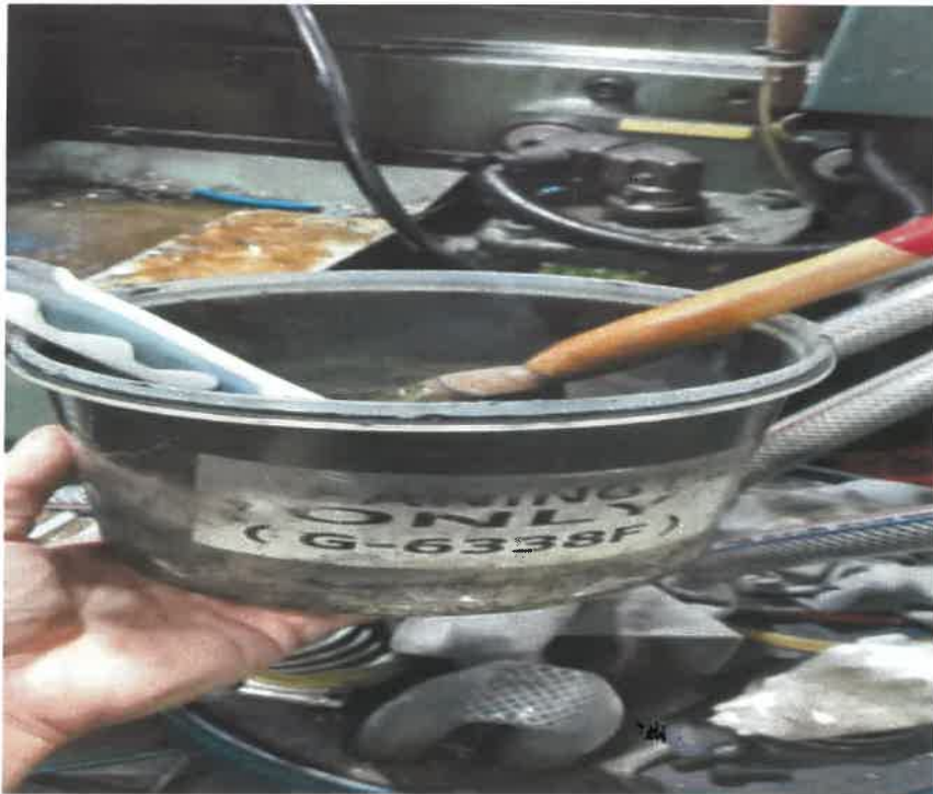
Figure 2.4.4 : Cleaning DIE bucket with toothbrush and huge brush with punching oil as lubricator
