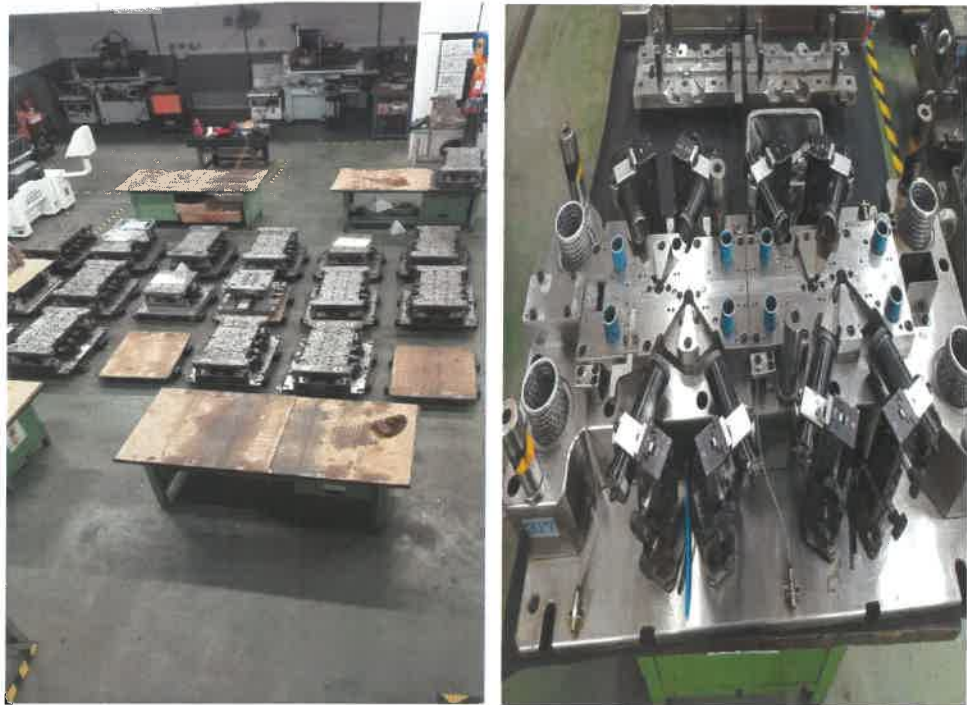
Figure 2.4.15 : Sample of DIE that need to be grind
