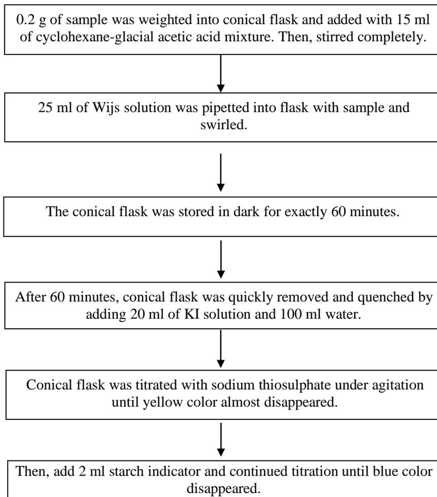
Figure 1 Process Flow of Iodine Value Determination.
