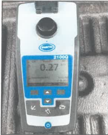
Figure 4 : HACH 2100Q (turbidity test)
