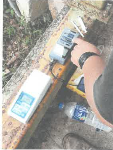
Figure 20: Turbidity and pH test.
