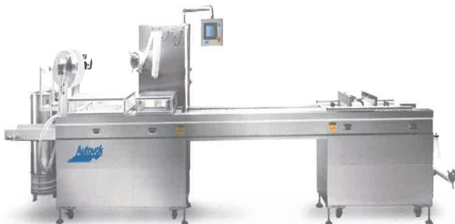
Figure 15: Form-fill seal machine
